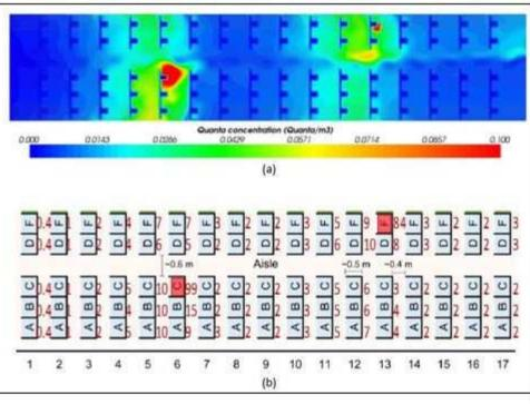
CFD output produced by SMARTFIRE coupled to Wells-Riley equation to produce probability of infection as a function of seat location. Two index patients are located on the train located in seats 6C and 13F, the carriage has an air exchange rate of 15 ACH. The index patients are emitting 14 quanta/hour through normal respiration.
